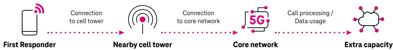
When a critical service worker's device tries to establish a radio connection to a nearby cell tower, priority access and preemption prioritizes that connection over others using information in that device's SIM card settings. Next, the prioritized device connects from the tower to the core network. Wireless Priority Service (WPS) prioritizes the traffic again, moving it to the front of the line if network restrictions exist.
